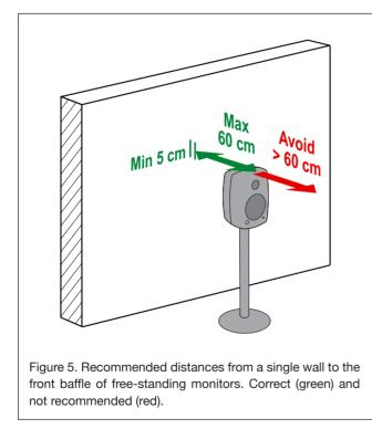
necessary when the monitors are placed near room boundaries. The attenuation levels are -2 dB, -4 dB and -6 dB.
