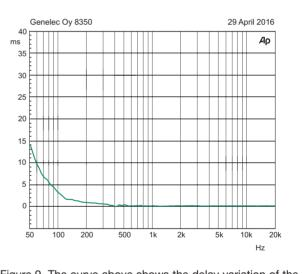
Figure 9. The curve above shows the delay variation of the 8350A as a function of frequency.
