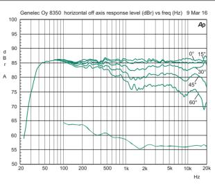
Figure 8. The upper curve group shows the horizontal directivity characteristics of the 8350A measured at 1 m. The lower curve shows the system's power response.
