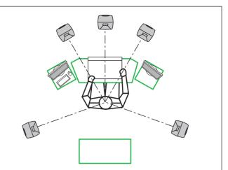
Figure 4. Symmetrical layout and keeping the acoustic axis clear from obstructions minimizes reflection surfaces and maintains accurate localisation because reflections are symmetrical.
