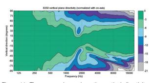
Figure 11. The curves above show the vertical directivity characteristics of the 8350A.
