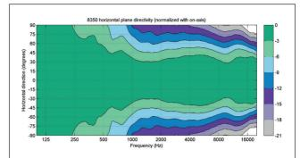
Figure 10. The curves above show the horizontal directivity characteristics of the 8350A.
