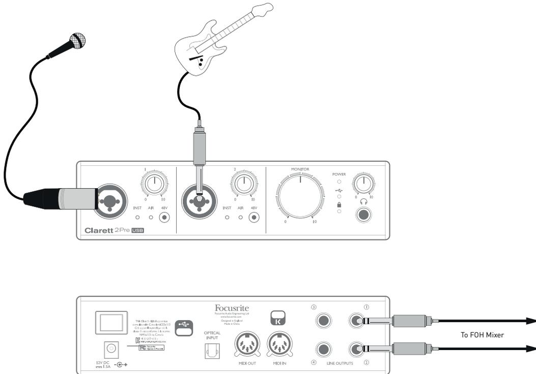
In the example illustrated, a mic and a guitar are connected to the inputs of the Clarett 2Pre USB; Outputs 1 and 2 go to the main PA system. The performer can adjust the volume of the mic and guitar separately from the front panel.
