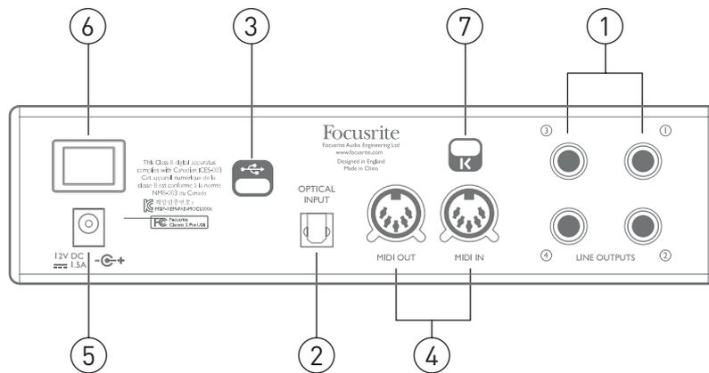
1. **LINE OUTPUTS 1 to 4** – four balanced analogue line outputs on 1/4" jack sockets; use TRS jacks for a balanced connection or TS jacks for unbalanced. Line Outputs **1** and **2** will generally be used for driving the main L and R speakers of your monitoring system, while Outputs **3** and **4** can be used for connecting additional line level equipment (e.g., outboard FX processors). The signals routed to all the outputs may be defined in Focusrite Control.
