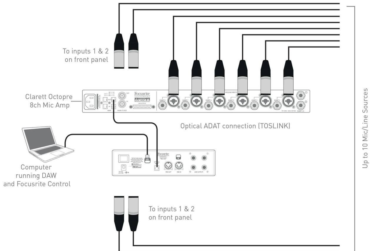
The Clarett OctoPre’s **OPTICAL OUT** port is connected to the Clarett 2Pre USB’s **OPTICAL IN** port with a single TOSLINK optical cable. The two devices must be synchronised to ensure audio passes cleanly, without clicks and pops. This can be achieved by selecting ADAT as the clock source in the **Device Settings** tab within the Focusrite Control software. Both devices must be set to the same sample rate.”
