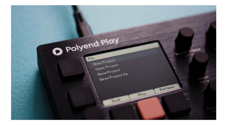
Each time you toggle the device on, Play boots to the last active project. All the currently active project changes are autosaved with each press of the Stop screen button. Projects can be loaded, and managed from the File menu level. Click the encoder to enter the file browser with the following options available:
