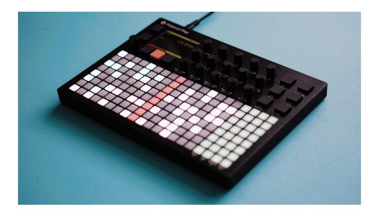
Each **track** is defined by a single horizontal row of grid pads. Each pad of the 16 leftmost columns represents a single **step**. The timeline/playhead advances from left to right and triggers steps containing data.
