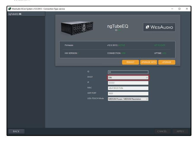
Before transitioning from a USB connection to Ethernet, it's crucial to configure the appropriate IP address on your ngTubeEQ. This setup ensures seamless communication between the device and your network. The subsequent chapter will guide you through the process of establishing the correct IP settings.
