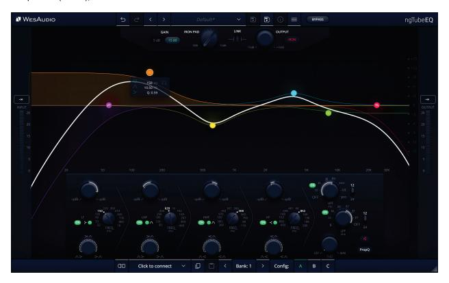
The layout of the mono plugin closely mirrors that of the hardware, maintaining the intuitive interface and design of the 2-channel stereo plugin version. However, there's a notable difference: the unit mode buttons (DUAL / STEREO / MS) are absent in this configuration. This is because, in mono plugin mode, the ngTubeEQ automatically operates in DUAL unlinked mode, optimizing it for independent channel processing.
