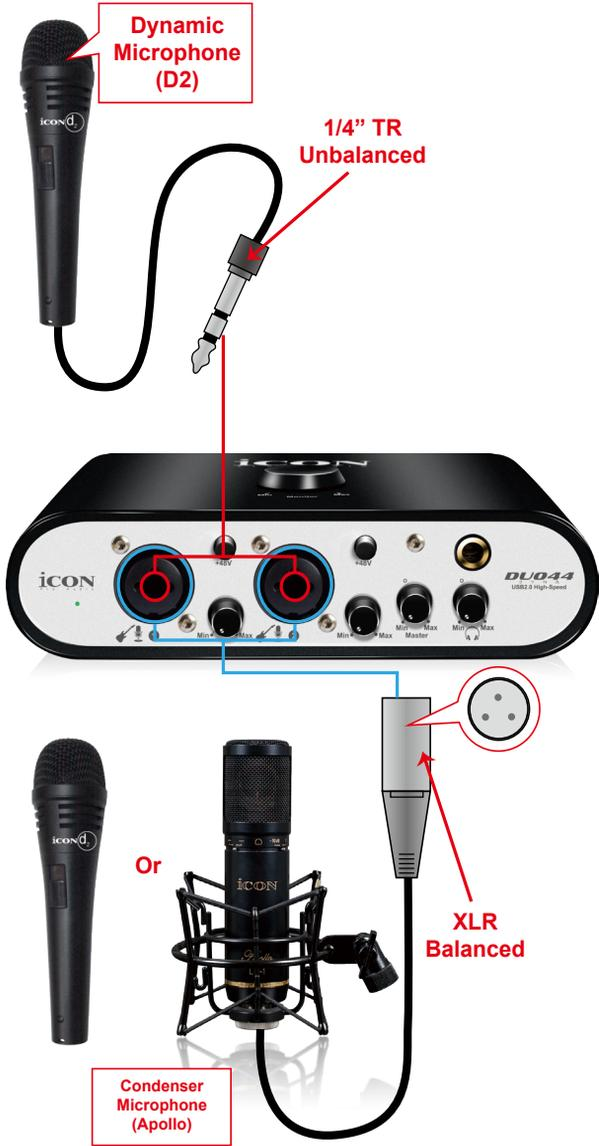
**Note:** For dynamic microphone user, please make sure +48V phantom power switch is "OFF" before you plug in your microphone, otherwise it may cause damage to your microphone.
