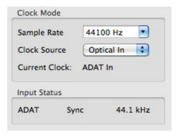
RME's exclusive **SyncCheck** technology (first implemented in the Hammerfall) enables an easy to use check and display of the current clock status. *SyncCheck* indicates whether there is a valid signal (Lock, No Lock) for each input (Word Clock, ADAT, AES), or if there is a valid *and* synchronous signal (Sync). In the field *Clock Mode* the clock reference is shown. See chapter 35.1.
