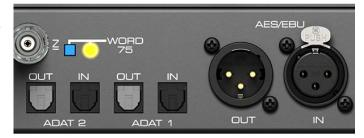
**ADAT2 I/O.** TOSLINK. Standard ADAT optical port, 8 channels. Can also be used as optical SPDIF input and output, if set up accordingly in the Settings dialog.
