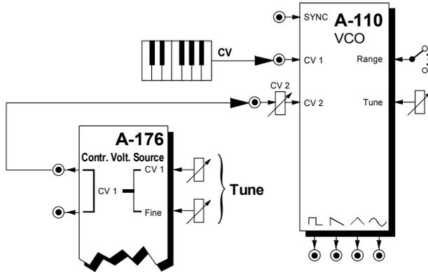
Fig. 2: Coarse and fine tuning an A-110 VCO.
