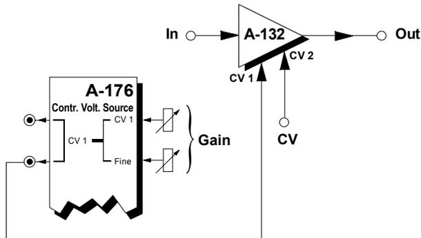
**Fig. 1:** Providing gain control for an A-132 VCA.
