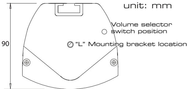
Top View of Column Loudspeaker with lid off
