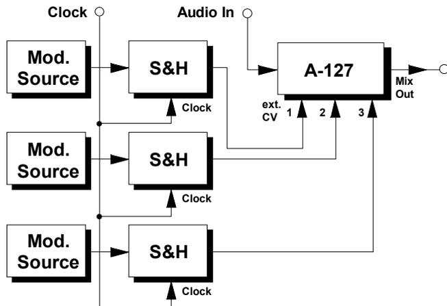
fig. 3: S&H filter effects with an A-148
