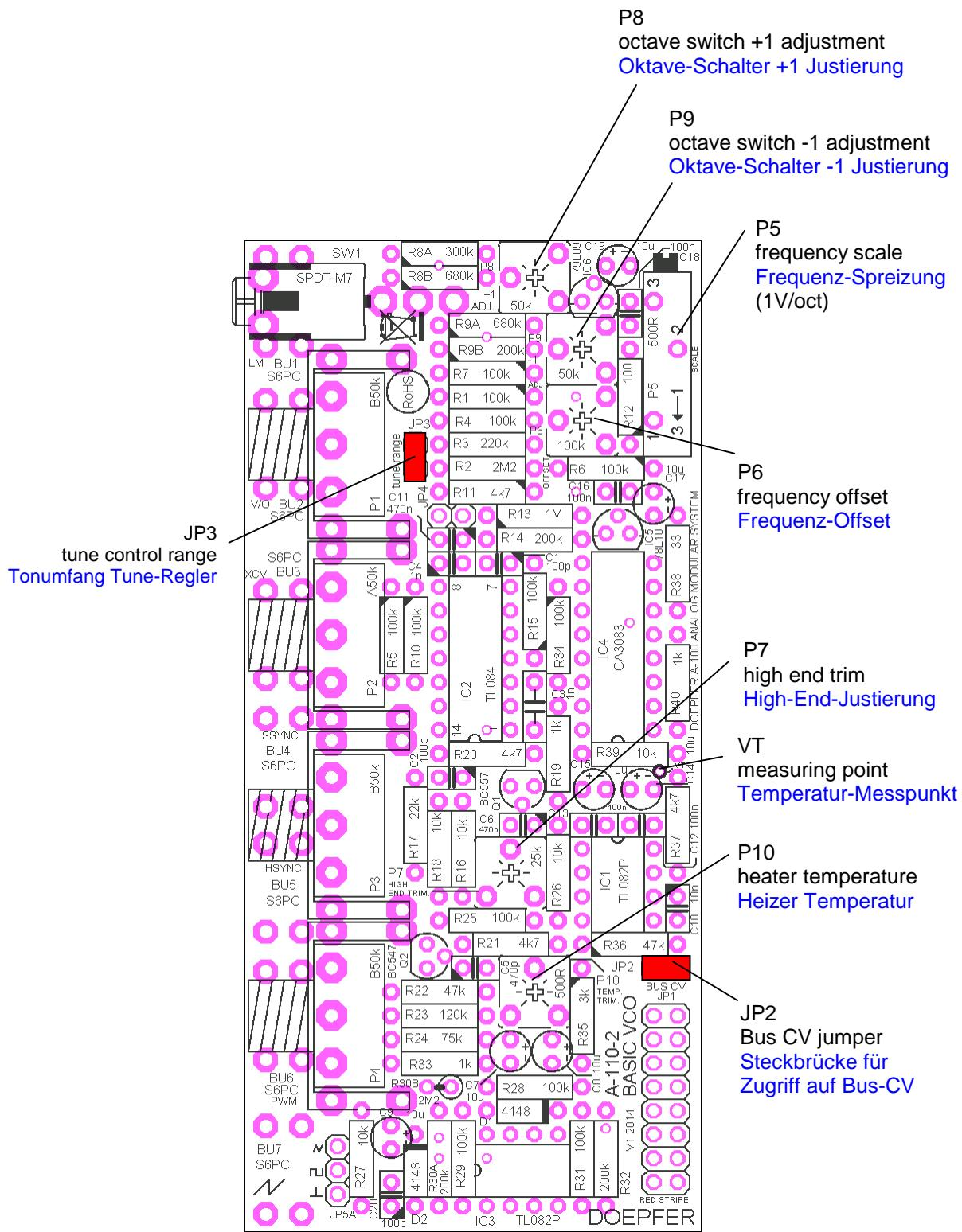
Temperature adjustment: P10 has to be adjusted to about +0.62V against GND at the measuring point VT (internal temperature adjustment of the VCO heater to about 50 degrees Celsius)
