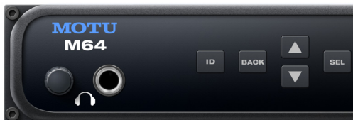
Figure 6-2: The volume knob is a push-button digital rotary encoder.
