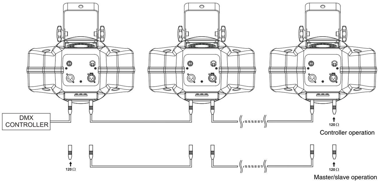
The fixture is equipped with 3-pin XLR sockets for DMX input and output. Only use a shielded twisted-pair cable designed for RS-485 and 3-pin XLR-plugs and connectors in order to connect the controller with the fixture or one fixture with another.
