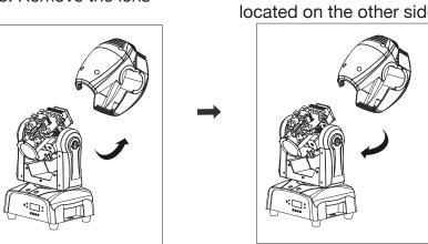
4. Unscrew the 4 screws located on the other side
