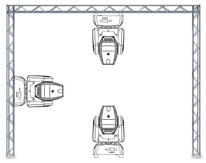
The Focus Spot One is fully operational in three different positions, hanging upside-down from a ceiling or trussing, mounted sideways on trussing, or set on a flat level surface. Be sure this fixture is kept at least 0.5m away from any flammable materials (decoration etc.). Always use and install the supplied safety cable as a safety measure to prevent accidental damage and/or injury in the event the clamp fails (see next page).
