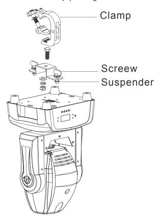
Screw one clamp via a M12 screw and nut to the included bracket. Attach the bracket using the omega locks to the bottom of the Focus Spot One. Attach and pull the safety-cable through one of the safety holes located on the bottom base and over the trussing system or a safe fixation spot. Insert the end in the carabine and tighten the safety screw.
