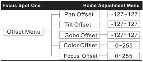
To enter the Offset Menu, press the MENU button to unlock the display, then press the ENTER button for at least 5 seconds. In this submenu you are able to adjust the home position of the pan, tilt, gobo wheel, color wheel, and focus. To exit this menu press and hold the MENU button.
