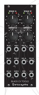
These are inputs of the second mixer (B) Scale A and Scale B knobs adjust attenuation/boosting/ inverting levels for each mixer output. At 12 o'clock there will be no signal on SCL output. Turning the knob clockwise, the signal level will increase until it's boosted to gain 2. Turning the
