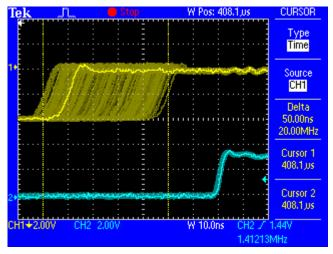
The cleaned and jitter-freed signal can be used as reference clock for any application, without any problem. The signal processed by SteadyClock is of course not only used internally, but also available at all outputs.
