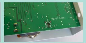
Using a small flat screwdriver set the initial gain of the pedal.
