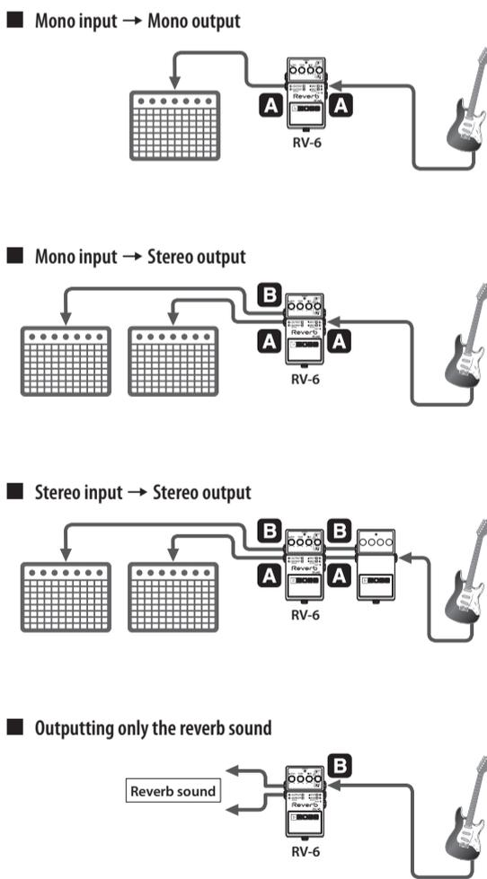
By plugging into INPUT-B, you can have only the reverb sound be output (the direct sound is not output).
