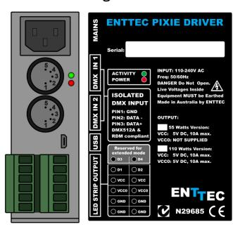
Pixie driver supports any kind of DMX output device. Here is a reference diagram of connections.
