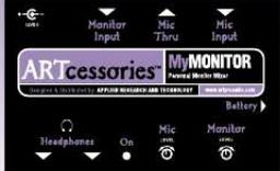
**Problem:** A performer needs to hear him/herself through headphones exclusively or mixed with the output of a mixer, CD player, tape deck, or other stereo line level source. Only the mic signal, however, should be going to the main mixer.
