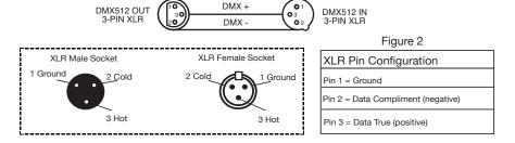
**Special Note:** Line Termination. When longer runs of cable are used, you may need to use a terminator on the last unit to avoid erratic behavior. A terminator is a 110-120 ohm 1/4 watt resistor which is connected between pins 2 and 3 of a male XLR connector (DATA + and DATA -). This unit is inserted in the female XLR connector of the last unit in your daisy chain to terminate the line. Using a cable terminator (ADJ part number Z-DMX/T) will decrease the possibilities of erratic
