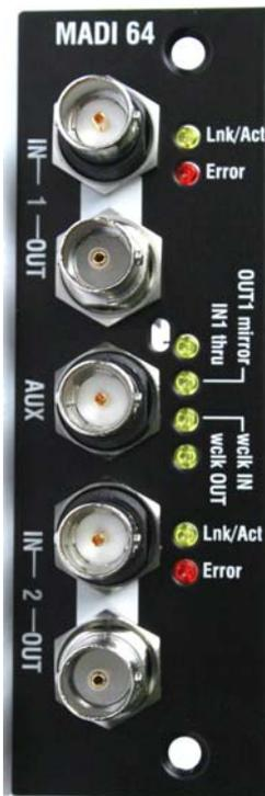
**M-MADI** is one of several plug-in card options that may be fitted to the iLive Series. It provides a multi channel digital audio network that can distribute signals between iLive and 3<sup>rd</sup> party MADI equipment. **MADI** offers an addition or alternative to EtherSound and other networking standards available for the iLive system.
