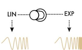
If the toggle is set to the left position, the FM signal will apply with linear scaling.
