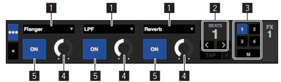
Single FX mode: One effect can be selected per effect unit and there are multiple adjustable parameters.
