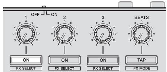
The effect switches between on and off each time the button is pressed.
