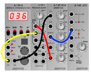
In this application the A-185-2 is used to add up several voltages that are used to control the pitch of all VCOs that are connected to the same bus board as the A-185-2:
