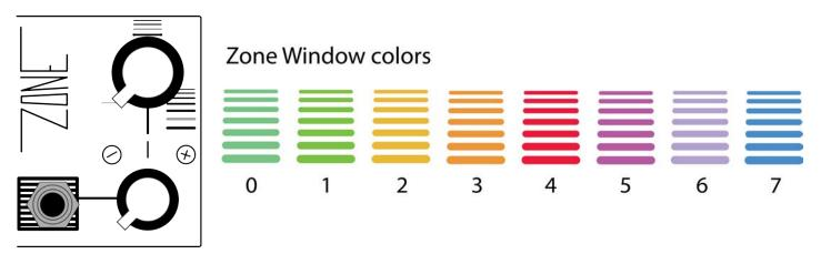
Switching Zones via the Zone control allows for large and instantaneous changes in repeat size without doppler/pitching effects, allowing quick smooth access to repeat sizes from microsound (shorter than 2 milliseconds) to phrase length (as long as 41 seconds).
