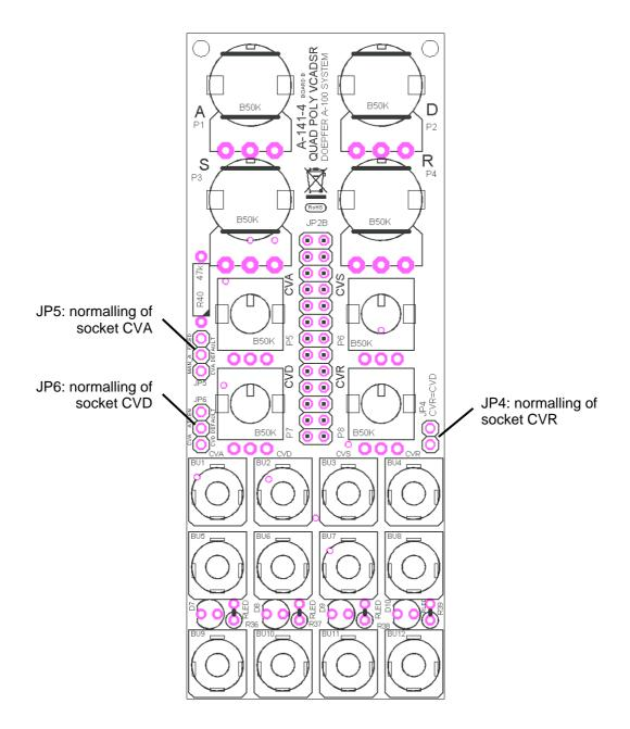
The pin headers JP4, JP5 and JP6 may be used for the normalling of the sockets CVA, CVD and CVR
