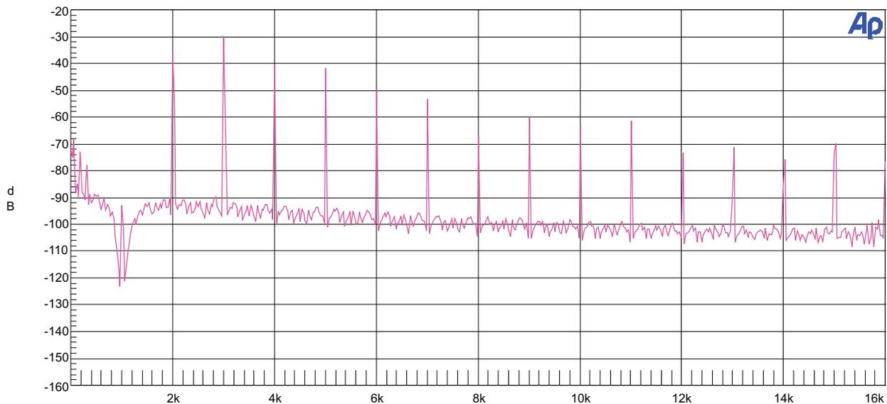
The TOP graph shows the distortion harmonics just prior to full clipping. Notice both even and odd harmonics and a smooth decay of upper harmonics.
