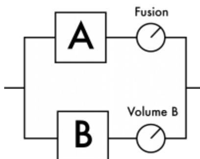
The Cold Fusion puts the Channels A and B in parallel. In other words, you will be able to adjust the level of Channel A that will be added to the output of Channel B. This technique consisting in adding a clean signal to a more distorted one is widely used in the studio to regain dynamics and articulation when the dirty sounds can be too compressed for example. The Fusion knob must be carefully adjusted and we recommend starting very low on this value and increasing gradually.
