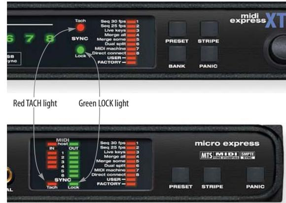
Figure 8-2: Converting time code. When your Express interface converts incoming time code, the red TACH light blinks, the green LOCK light glows steadily, and the green Computer I/O light glows steadily as well.
