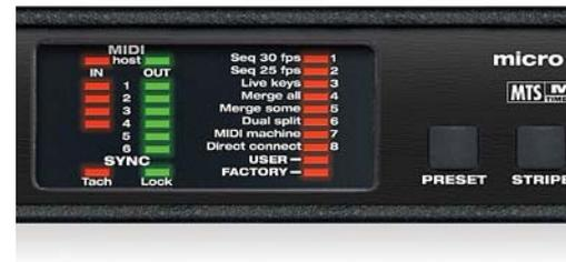
Figure 7-1: The eight factory presets on the front panel of the Express XT and micro express.
