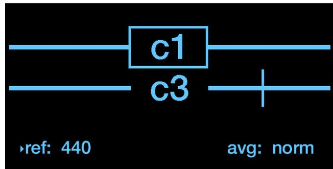
A note is sharp if the vertical line is to the right of the note name. For example, in this illustration the vertical line is to the right of the note name for CH 2, indicating that CH 2 is playing a C3 ("middle C"), but that the note is sharp.
