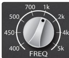
**Mid Band Frequency.** Sets the center frequency of the EQ's mid-frequency band. You can adjust the center frequency between 400 Hz and 5 kHz.
