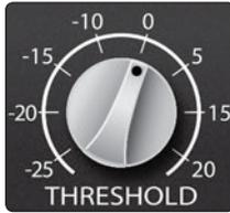
**Threshold.** Sets the threshold of the compressor. When the signal's amplitude (level) exceeds the threshold setting, the compressor engages. Turning the knob counter-clockwise lowers the threshold so that compression begins at a lower amplitude, and more of the input signal is compressed. The threshold can be set from -25 to +20 dBu.
