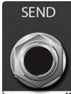
**Balanced Send.** This balanced 1/4" TRS output sends the source signal out of your RC 500 before the compressor, EQ, and Master Gain stages. Use this output to insert an external processor into your RC 500's signal path.
