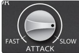
**Attack.** Attack sets the speed at which the compressor acts on the input signal. A slow attack time (fully clockwise) allows the beginning component of the signal (commonly referred to as the initial transient) to pass through, uncompressed, whereas a fast attack time (fully counter-clockwise) triggers compression immediately when a signal exceeds the threshold. The compressor attack time ranges from 0.5 ms (Fast) to 10 ms (Slow).
