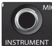
**Instrument Input.** The 1/4" TS connector on the front panel is for use with a passive instrument (guitar, bass, etc.). To use this input, turn the Source Select switch to the Mic/Inst position.
