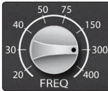
**Low Band Frequency.** Sets the center frequency of the EQ's low-frequency band. You can adjust the center frequency between 20 and 400 Hz.
