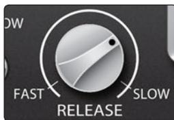
**Release.** Sets the release of the compressor, which is the time the compressor takes to return the gain reduction back to zero (no gain reduction) after the signal level crosses below the compression threshold. The compressor release time ranges from 40 ms (Fast) to 500 ms (Slow).
