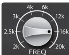
**High Band Frequency.** Sets the center frequency of the EQ's high-frequency band. You can adjust the center frequency between 2 and 20 kHz.
