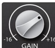
**High Band Gain.** Sets the attenuation or boost of the EQ's high-frequency band. The gain can be set between -16 and +16 dB.
