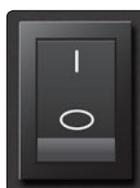
**Power Switch.** Turn this switch to the [I] position to power on your RC 500. The [O] position powers the unit down.
