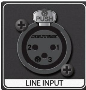
**Line Input.** This balanced XLR connection can be used for line-level devices such as keyboards, drum machines, and sound modules. To use this input, turn the Source Select switch to the Line position.
