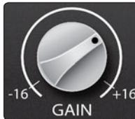
**Low Band Gain.** Sets the attenuation or boost of the EQ's low-frequency band. The gain can be set between -16 and +16 dB.
