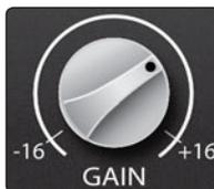
**Mid Band Gain.** Sets the attenuation or boost of the EQ's mid-frequency band. The gain can be set between -16 and +16 dB.
