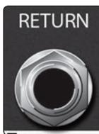
**Balanced Return.** This balanced 1/4" TRS input patches directly to the compressor stage of your RC 500. When using this input to insert an external dynamics processor, you can bypass the compressor, the EQ, or both.
