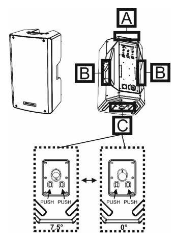
A –Upper integrated handle B – Lateral integrated handles C – Pole mount hole, with two tilt angles
