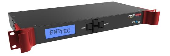
ENTTEC'S PIXELATOR is a 24-port Ethernet to pixel controller. Using ENTTEC'S PLINK protocol, each port provides data to ENTTEC'S PLINK INJECTORS which can output up to 2 Universes each. The Pixelator can send data up to 24,576 channels (8,192 RGB pixels) with perfect synchronization across all eight of its outputs.
