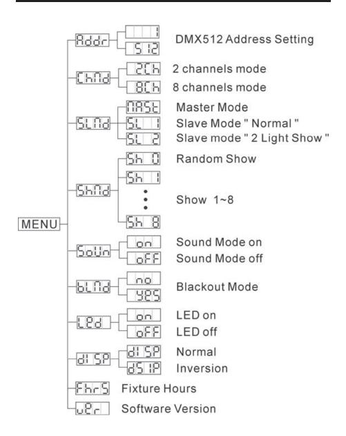
**n-Board System Menu.** The Majestic LED comes with an easy to navigate system menu. This next section will detail the functions of each command in the system menu. **Please read the next section thoroughly!**
