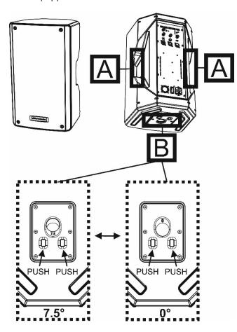
A - Lateral integrated handles B - Pole mount hole, with two tilt angles selection (0°/ 7.5°)
