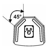
The rear side inclination, symmetrical, as shown in the upper picture, is 45°. KL10 can be used as a stage monitor in small contexts, in this case please consider the characteristic dispersion pattern presented above.
