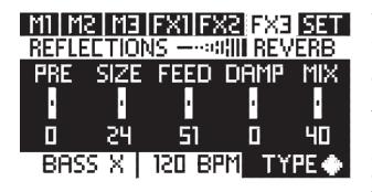
While on the main page, rotating the encoder, will make a swap between the pages, but while in a menu, where you have lists, it will scroll the list. For a better view over that, you can also check the image located on the quick start guide.
