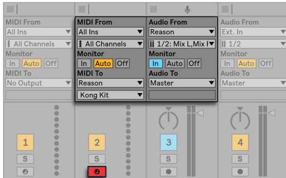
An Audio Track Receiving Audio From and a MIDI Track Sending MIDI to Reason.
