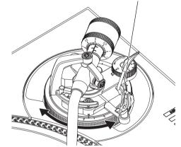
Refer to the following table to adjust the [HEIGHT ADJUST] dial to match the height to your cartridge size.
