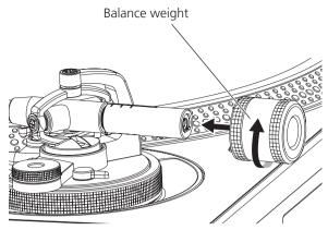
When using a cartridge between 9.5 g and 13 g, attach the sub weight on the rear shaft of the tone arm. ٠
