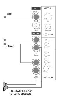
If your source provides bass management, you can use the BM9S II LFE input alone in LFE or SLAVE mode, depending on the management system capabilities. Avoid double processing if possible.
