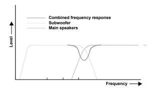
With the phase settings you can adjust the phase relationship between the subwoofer and main speakers. If either subwoofer or main speaker are slightly out of phase in relation to the other, it can result in decreased bass output in the frequency response area where they overlap each other.
