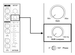
The SUB Lowpass control allows the frequency range of the subwoofer to be defined. Above the selected frequency the sound level decreases rapidly. The correct setting of this cut-off frequency is important for a well balanced combination of subwoofer and speakers.
