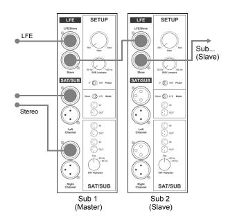
The BM9S II can be used stand-alone or together with multiple subwoofer units. Using multiple units may be helpful if the listening room is quite large or has difficult acoustic conditions. When using two or more subwoofers, the first one (designated "Master") controls the following subs (designated "Slave") via a subwoofer cable.
