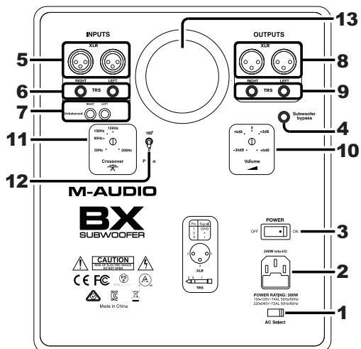
4. **Subwoofer Bypass:** Connect the included footswitch to this input, and then use the footswitch to momentarily bypass the low frequencies generated by the subwoofer (including the amp, driver, and crossover), sending the full-bandwidth signal directly to your main monitors. This lets you conveniently audition mixes with and without the low-frequency extension of the subwoofer. The **LED Indicator** on the front of the subwoofer flashes **red** when in Bypass Mode.
