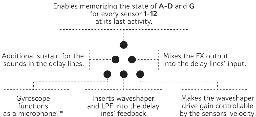
\* A unique mode where the built-in Gyroscope acts as a microphone with very special characteristics, picking up sound from TERRA's body.
