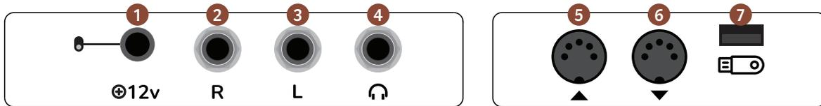
**1 12 volt DC input**, 0.4A, "+" in the center, 5.5 x 2.1 mm; and the power switch connected to it. TERRA comes with a high-quality power supply. In case of losing it, use a high-quality modern switching power supply with corresponding parameters!
