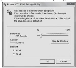
A sufficiently large buffer size decreases the chance of sound dropout (sound interruption) but increases audio signal transmission delay (latency).
