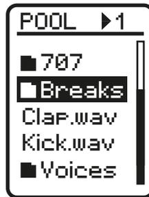
This can be thought of as an additional 'load only' folder for storing bulk or uncategorised samples to browse through when designing banks directly on the Squid. Squid will automatically create a Pool directory on start up if a folder does not already exist.
