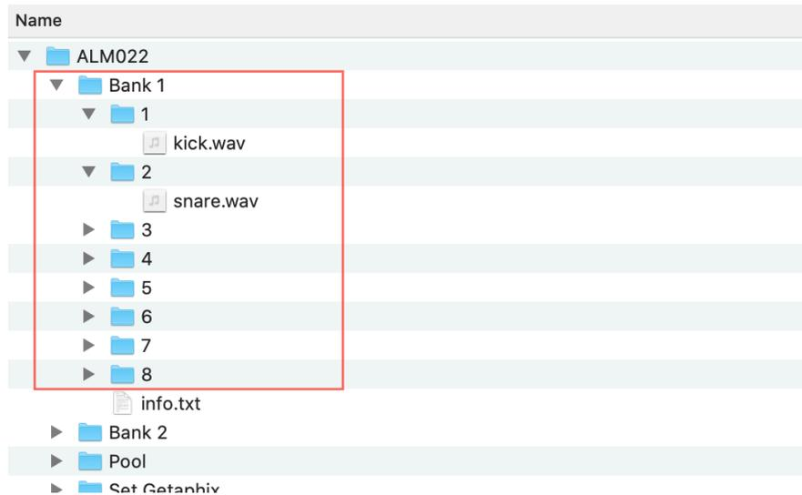
(Note if a numbered directory does not exist squid will fall back to loading a file named Chan-00x.wav with x being the channel number - this ensures compatibility with earlier firmware releases).
