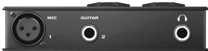
Figure 4-2: MicroBook front panel
