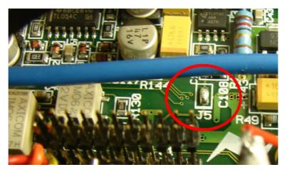
Shown above, the module set to work in Standalone mode before the modification has been made. All 1073LB Mic Pre modules leave the factory set to work in Standalone mode.
