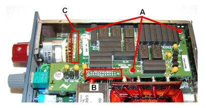
► Gently prise the top board off its 20-pin connector (**B**) taking care not to disturb the ribbon cable fitted under the far left of the board (**C**).
