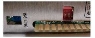
Shown above, the module set to work in insert mode after Switch 2 has been changed from the factory default.
