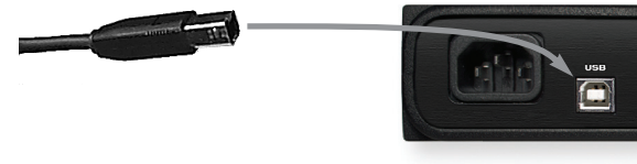
Figure 2-2: The square Type B plug goes into your MOTU interface.
