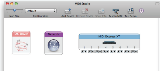
Figure 3-1: In this example, a MOTU MIDI Express XT interface as it appears in the MIDI window of Audio MIDI Setup.
