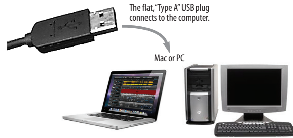
Figure 2-1: You can plug the Type A connector directly into the computer itself, a USB keyboard connected to the computer, or any other USB device already connected to the computer that has an available Type A USB jack.
