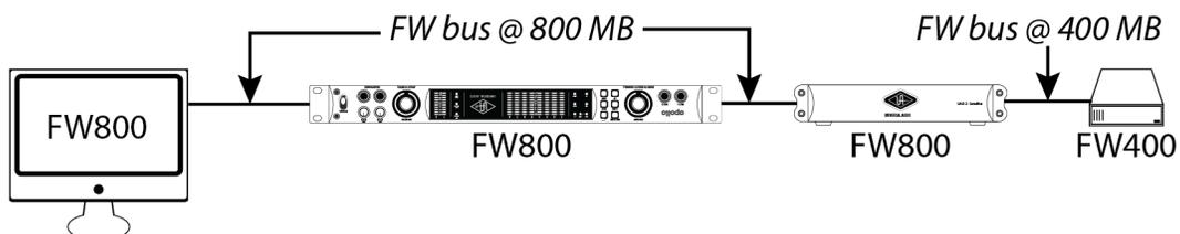
*This FireWire bus runs optimally at both 800 megabits and 400 megabits because the FireWire 400 device is located AFTER the FireWire 800 devices in the setup.*
