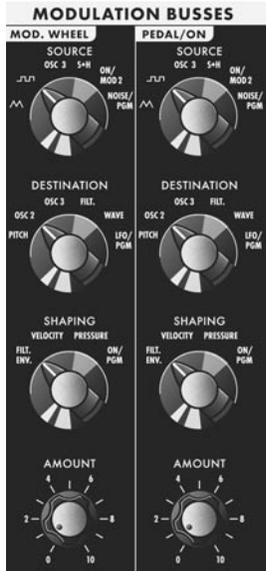
The Modulation Busses allow you to select a variety of modulation sources, destinations, modulation shaping, and amounts. The two Mod Busses are labeled MOD WHEEL and PEDAL/ON. The performance control for the MOD WHEEL Buss is the Modulation Wheel itself, while the performance control for the PEDAL/ON Buss is the MOD 1 Input jack on the Patch Panel.
