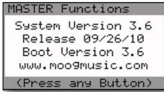
The SOFTWARE VERSION screen displays the current Operating System ROM and BOOT ROM versions and date of the release.
