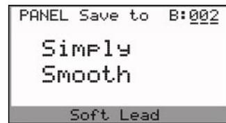
When EDIT is selected, the bank and memory location defaults to the last saved location. For example, if the last saved location is G009, the default EDIT memory location will be G009 as shown. Note also that the name of the Preset that is stored at the specified memory location is always displayed, preventing you from accidentally overwriting a special preset.
