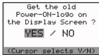
The POWER-ON SCREEN function allows you to select the original Voyager Power-on logo or the new XL Power-on logo. To change the appearance of the Power-on screen, use the **CURSOR** to select 'YES' and press **ENTER**. To leave this menu without changes, select 'NO' and press **ENTER**.
