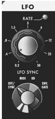
To generate the S+H function, the LFO's square wave is used as the S+H Trigger, while the Voyager XL Noise source is used for the S+H Input signal. For each positive-going cycle of the LFO square wave, the voltage at the input of the S+H circuit is sampled and held until the next cycle. Since the sample source is Noise (a random signal), the voltage that appears at the output of the S+H circuit is a random voltage that changes in time with the LFO.
