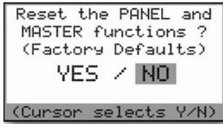
The FACTORY RESET function resets the Voyager PANEL and MASTER functions to the default factory state (see list of default values below). To reset the PANEL and MASTER functions select 'YES' and press **ENTER**. To escape without restoring the Factory presets, select 'NO' and press **ENTER**.
