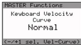
The VELOCITY CURVE function allows you to tailor the velocity response to your playing style. The Voyager XL offers three velocity curves: SOFT, NORMAL, and HARD. SOFT achieves high velocity values with a light touch. NORMAL is the unprocessed velocity curve of the Voyager XL Keyboard. HARD requires a heavy touch to achieve high velocity values. To change this setting, use the **-1/+1** buttons to select the desired Velocity Curve.
