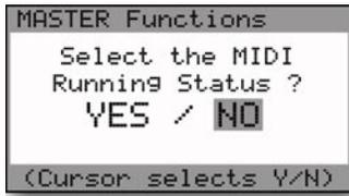
The MIDI RUN STATUS (MIDI Running Status) function is used to reduce the MIDI data sent when a number of MIDI messages with the same Status Byte are sent. When enabled, the Running Status function eliminates the Status Byte. Some MIDI devices can handle MIDI Running Status and some can't, so you have an option of turning this on ('YES') or off ('NO'). To change the setting, use the **CURSOR** to highlight the desired choice and press **ENTER**.
