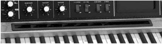
The 500mm Ribbon Controller is located on the middle wooden rail of the Voyager XL. The Ribbon's center point is lined up with 'Middle-C' on the 61-note keyboard. The Ribbon can be used to impart complex gestures to a given sound by touching the ribbon, by moving a
