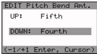
The PITCH BEND AMT function allows you to set separate up and down pitch bend ranges for each preset. To adjust the ranges, use the **CURSOR** to toggle between the Pitch Bend UP and Pitch Bend DOWN parameters, and use the **-1/+1** buttons to select the desired range.
