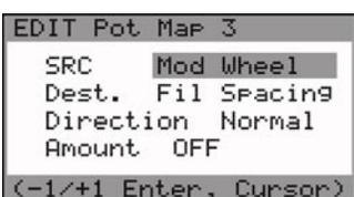
A new menu will appear, similar to the one shown at left for Pot Map 3. All four map menus are identical and have the same assignable options. The menu allows you to select the source (SRC), the destination (DEST), the direction, and the amount for each of the four mappings. Use the **CURSOR** to move to the desired parameter; then use the **-I/+I** buttons to select the desired value.
