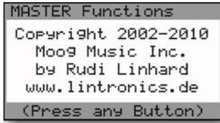
The COPYRIGHT INFO screen shows the copyright dates, as well as the creator of the Voyager's operating system, Rudi Linhard. This is also the entry page to the Factory Setup menus – simply press the **+1** button to view the Factory Setup Menu.
