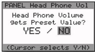
HEADPHONE VOLUME is used to determine whether the stored Headphone Volume value is loaded when a new preset becomes active. If this is off, then this value is determined by the current position of the **HEADPHONE VOLUME** control. To make a change in the Headphone Volume menu, use the **CURSOR** to highlight the desired choice and press **ENTER**.
