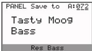
The SAVE PRESET function allows you to store all of the current front panel settings and software parameters to one of the available 896 memory locations.
