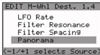
PGM M-WHL DEST allows you to program one of 8 additional modulation destinations to be used when the Mod Wheel Mod Bus **DESTINATION** control for the set to 'LFO RATE/PGM'. To select a destination, use the **-1/+1** buttons to highlight the desired selection and press **ENTER**.
