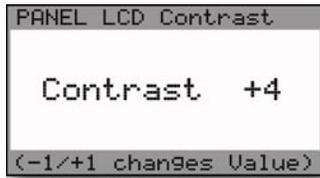
The LCD CONTRAST function changes the viewable angle of the LCD display. To change this setting, use the **-1/+1** buttons to adjust the contrast level. The change will immediately take effect (you'll see the display contrast change) and the new contrast value will be stored automatically.
