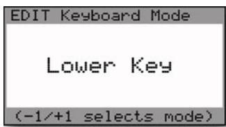
KEYBOARD MODE allows you to select one of 4 types of keyboard priority for a preset. The keyboard priority determines what happens when more than one key is pressed on the keyboard. To set the Keyboard Mode, use the **+/-I** buttons to select one of the following options:
