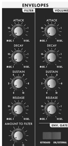
When triggered, EG's produce a time-varying control voltage that has a specific start, middle and end profile. The parameters that define this CV profile are Attack, Decay, Sustain and Release, sometimes abbreviated as ADSR.
