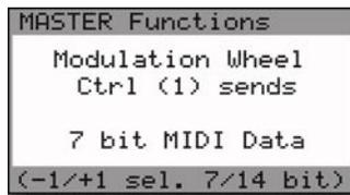
The MIDI Modulation Wheel function allows you to select the transmission of 7-bit or 14-bit MIDI Control Change (CC) messages from the Mod Wheel. Use the **-I/+I** buttons to change the setting. In 7-bit mode, only MIDI CCI is sent when the Mod Wheel is moved. In 14-bit mode, both MIDI CCI (Most Significant Byte (MSB)) and MIDI CC33 (Least Significant Byte (LSB)) are sent when the Mod Wheel is moved.
