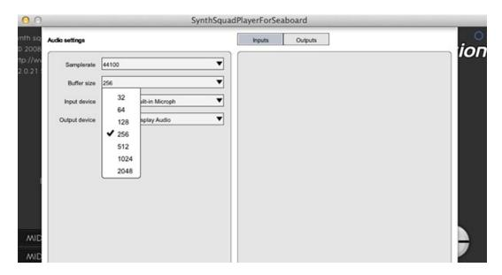
Because of its extensive sound engine Synth Squad is quite CPU intensive so in general the **buffer size should be set no lower than 256** and the sample rate should be set to 44100. These settings should give a low latency, high quality playing experience; however it does depend on the computer in use. If the audio output of Synth Squad begins to break up the buffer needs to be set higher.
