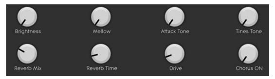
The eight Macro knobs control different sound parameters within the Synth Squad sound engine. Control them with a mouse, or with a standard MIDI controller using the MIDI Learn function. Since each preset has different sounds attributes (e.g. decay, chorus, tone, etc) the Macro parameters are always unique and change from preset to preset.
