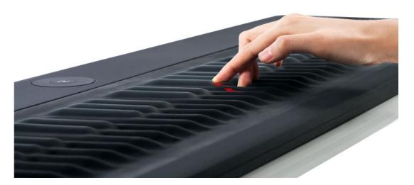
The Seaboard interprets the playing of two adjacent notes in succession (C  $\rightarrow$  C #), as pitch bend. This is achieved via a smooth legato gesture, varying the pressure during the duration of the gesture. It's possible to extend the pitch bend even further by continuing the legato gesture chromatically (e.g. simultaneously C  $\rightarrow$  C  $\# \rightarrow$  D  $\rightarrow$  D #)
