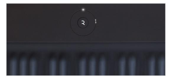
Synth Squad's preset structure can be navigated with the User Dial. The presets are divided into four banks of twelve: **A01-12, B01-12, C01-12, D01-12**. Pressing the Center Button will advance to the next bank in a clockwise direction. However, use the Control Ring to navigate through presets in either direction. Each full revolution of the Control Ring advances to the next bank.
