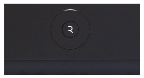
The **Octave Shift** mode transposes the Seaboard's playing pitch up or down. Hold down the Center Button until the Light Ring displays a wide band of light across the top center. Turn the Control Ring counter-clockwise to shift the pitch an octave down. Turn it clockwise to shift it up. The transpose range is two octaves and normal playing position is when the LEDs are centered. Press the Center Button to exit Octave Shift mode.
