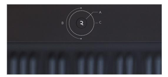
The **User Dial** is located on the top panel of the Seaboard. You can use it to navigate between presets of Synth Squad and other virtual instruments There are 3 elements to the User Dial: the Center Button, the Control Ring and the Light Ring.
