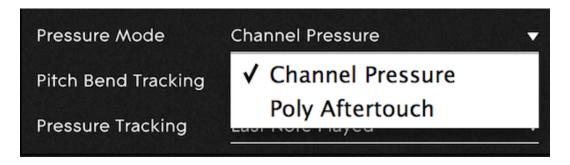
Pressure Mode will determine how changes in playing pressure are transformed into MIDI data. The options are **Poly Aftertouch** and **Channel Pressure**. Select Channel Pressure to affect all notes at once. Select Poly Aftertouch to give independent pressure control over individual notes.
