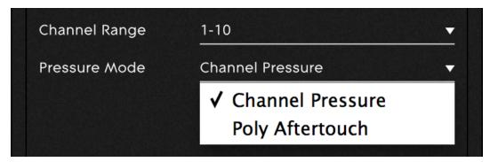
Pressure Mode will determine how changes in playing pressure are represented as MIDI messages. The options are **Poly Aftertouch** and **Channel Pressure**. Note that since in Multi- Channel mode each note is on a different channel, both options allow individual pressure control of each note.
