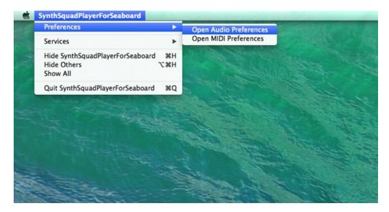
Choose the desired audio outputs. These can be either the built- in core audio outputs or outputs from a connected audio interface. The default buffer setting is 256. If you experience crackles in the audio try setting the buffer to a higher value.
