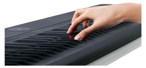
The Seaboard's ability to respond to continuous pressure is a powerful feature. Unlike traditional keyboard aftertouch, the continuous pressure control begins as soon as you touch the key. This results in a bigger physical range and a considerably higher digital resolution.
