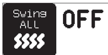
When SWING ALL is set to any value except OFF, the track parameter knob SWING controls the SWING ALL value.
