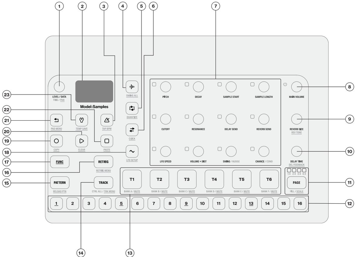
1. **LEVEL/DATA** sets the overall volume level of the active track. You also use it to set parameters and navigating menus. The secondary function sets the track pan. **[TRIG] + LEVEL/DATA** opens the TRIG NOTE menu.
