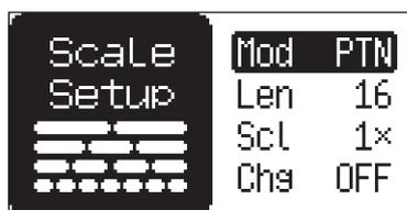
**MOD** Mode can be set to either PATTERN or TRACK. In PATTERN mode all tracks share the same SCALE and LENGTH settings. In TRACK mode, all tracks can have individual SCALE and LENGTH settings. Press [T1-6] to select the track to set the scale for.
