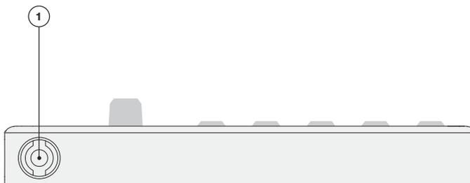
1. **BATTERY DC In**, Input for accessory battery power supply.
