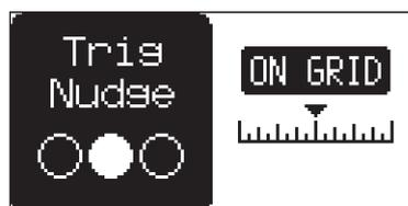
1. In GRID RECORDING mode, press and hold one or several **[TRIG]** keys and then turn **SWING** to access the TRIG NUDGE menu that shows the time offset for the chosen sequencer trig(s) on the active track.
