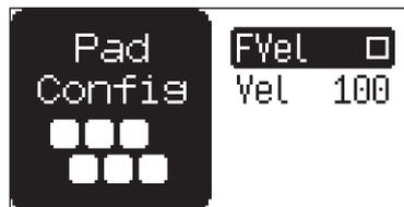
**FVEL** Fixed velocity set the pads to trig with a fixed velocity. (ON, OFF)
