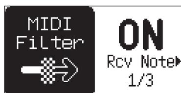
**RCV NOTE** will when active, make it possible to play Model:Samples using an external MIDI keyboard or controller.
