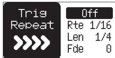
**ON/OFF** Toggles the retrigger function ON/OFF for the chosen trig.
