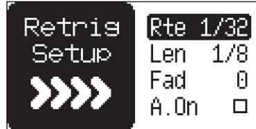
**RTE** Sets the retrigger rate (1/1, 1/2, 1/3, 1/4, 1/5, 1/6, 1/8, 1/10, 1/12, 1/16, 1/20, 1/24, 1/32, 1/40, 1/48, 1/64 or 1/80). 1/16 is the nominal retrigger rate, one trig per step. 1/32 corresponds to two trigs per step and so on. To trig triplets, for example, set the retrigger rate to 1/12 (or 1/24).
