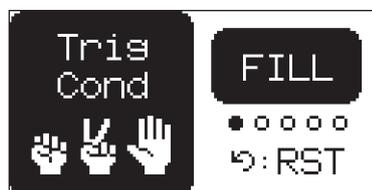
Conditional locks are a specific kind of Parameter locks. Conditional locks give you the possibility to set a number of conditional rules for any trig. These conditional rules are called Trig conditions. They are logical conditions that determines whether a trig set in the sequencer is triggered or not. If the condition is true, then the trig becomes active and affect the track.
