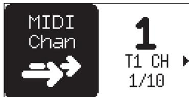
**T1–6 CH** selects the dedicated MIDI channel that is used to receive or send (by turning the knobs) parameter data to or from a specific track. If configured as OFF, parameter data are neither received nor sent via MIDI.
