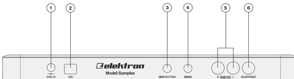
1. **DC IN**, Input for power supply. Use the included PSU-4 power adapter, connected to a power outlet.
